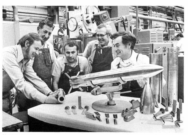
SCALE MODEL of weapon now under development was built for Structural Design Division 8157 for wind tunnel testing. It represents over 1500 hours of machining and is the work of (from left) design draftsman Bob Graham (8432) and machinists George Dawson, Andy Cardiel, Dell Houser and Bill Lavinsky of Machine Shop Section 8423-1. The intricate model has over 50 separate parts; Roger Everett is project engineer and Roger Page test engineer.
